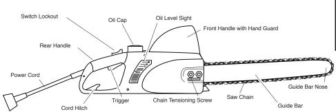
Figure 2 - Chain Saw Model 107624-02
